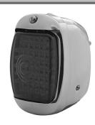
'37-'38 LED Tail Lights for Cars and '40-'53 LED Tail Lights for Trucks 45 super bright red LEDs for tail and 6 super white LEDs for license (on driver side). Red lens.
